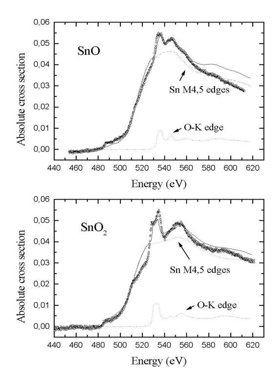
Figure 1. Comparison of EELS data (open circles) and calculations (solid line). Contributions of both tin and oxygen edges are also shown (as dotted lines). Upper panel: SnO, experimental resolution 2.6 eV. Lower panel: SnO<sub>2</sub>, experimental resolution 1.8 eV.
