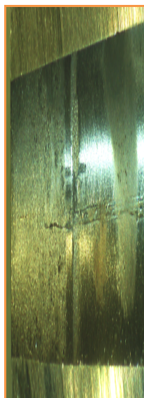
Figure 2. Photograph of wear damage on interior of housing
