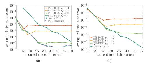
Figure 9.2. Model reduction results for tubular reactor of Kramer and Willcox (2019, Figure 6), showing the relative state errors for several different reduced models as a function of the reduced model dimension. Here  $\mathcal{D} = 0.167$ .
