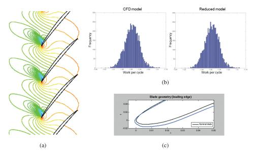
Figure 7.1. Model reduction results for compressor blade example of Bui-Thanh *et al.* (2008*b*). (a) Representative CFD pressure fields. (b) Histograms of work per cycle computed over 5000 different blade geometries using linearized CFD (n = 103008 dof) and a parametric POD reduced model (r = 307 dof). (c) Close-up of one sampled blade geometry compared to the nominal blade.
