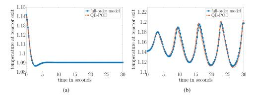
Figure 9.1. Model reduction results for tubular reactor of Kramer and Willcox (2019, Figure 5). The reduced model uses lifting to quadratic-bilinear (QB) DAE form,  $r_1 = 30$  POD modes to approximate the differential equations and  $r_2 = 9$  POD modes to approximate the algebraic equations. (a)  $\mathcal{D} = 0.162$  (stable case). (b)  $\mathcal{D} = 0.167$  (unstable case).
