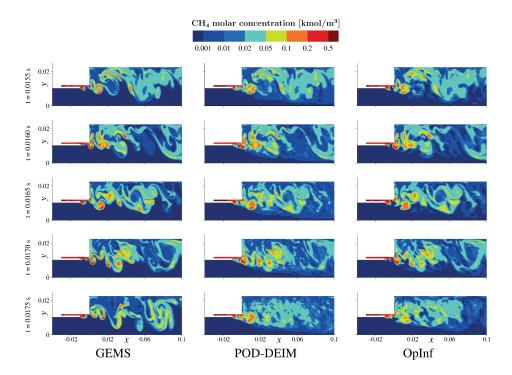
Figure 9.4. Model reduction results for the single-injector rocket combustion process of McQuarrie *et al.* (2021, Figure 8). Molar concentrations of CH<sub>4</sub> produced by GEMS (308 184 dof, left column), POD-DEIM (70 dof, middle column), and OpInf (43 dof, right column). POD basis computation and reduced model training used the first two milliseconds of data. (Figure reproduced with permission. Copyright © 2021 Taylor & Francis Ltd., www.tandfonline.com.)
