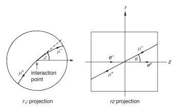
Fig. 11.8. Track reconstruction in a solenoid detector (shown for an event  $e^+e^- \rightarrow \mu^+\mu^-$ ).
