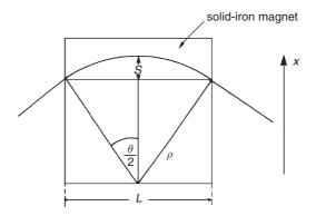
Fig. 11.5. Illustration of the sagitta method for momentum determination [4].
