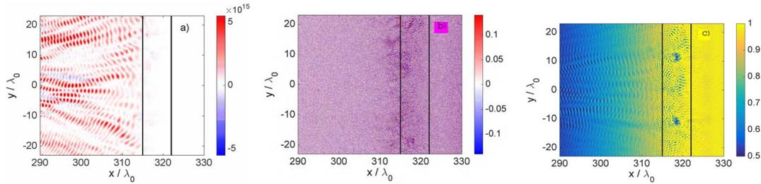
**Figure 7.** (a) Spatial distribution of the Poynting vector ( $x$ -component in  $\text{W}/\text{cm}^2$ ) in real space around the critical density, (b) the charge density  $(Zn_i - n_e)/n_c$  and (c) the ion density normalized to the critical density  $Zn_i/n_c$  for the laser pulse time  $t_p = 0$  and the simulation time  $t = 5$  ps. The solid black lines represent the region  $(0.9 - 1)n_c$  near the critical density.
