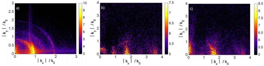
**Figure 5.** (a) Fourier spectra of electromagnetic waves, (b) electron plasma waves – charge density, and (c) ion acoustic waves in the quarter critical density region for the laser pulse time  $t_p = 0$  and the simulation time  $t = 5$  ps. Color bars are in logarithmic units.
