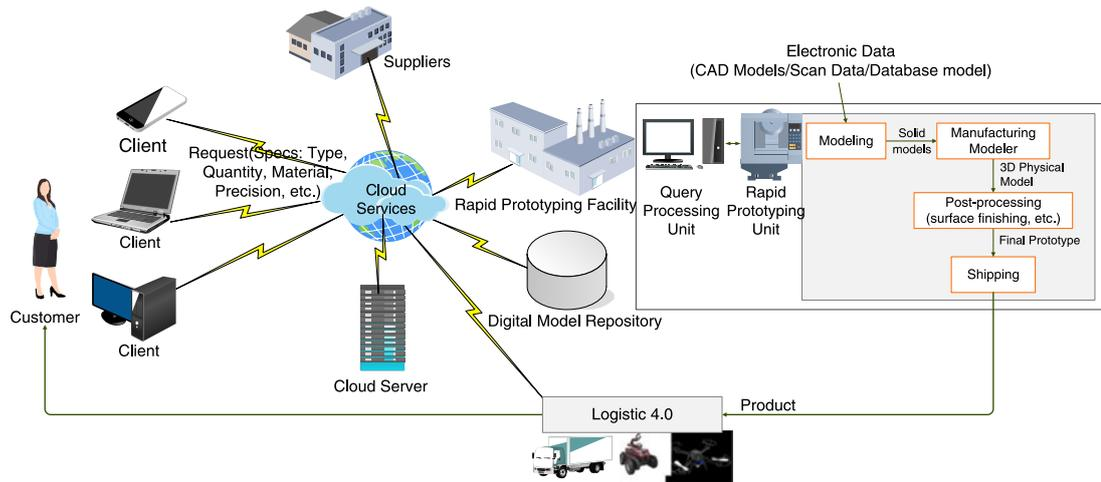
**Figure 3** Overview of the smart-rapid prototyping scenario
