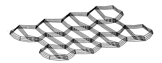
Fig. 8 DEFORMED SHAPE OF TOP SURFACE DUE TO FIGURING PRESSURE Fig. (8) shows the deformation of the top surface of the honeycomb when under the influence of Gravity and an estimated figuring pressure of 0.2 psi. The rear surface of the mirror was constrained in the vertical direction. The central cell of this section is representative of the majority of the cells in the mirror whilst the outer cells represent those near the edge of the mirror.
