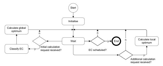
Figure 5. Logic architecture of the 'Optimiser Agent'
