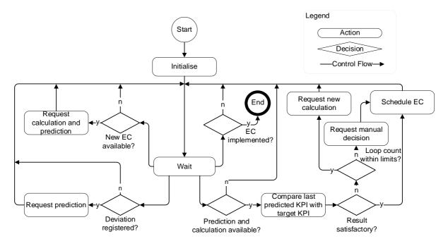
Figure 4. Logic architecture of the 'Negotiator Agent'
