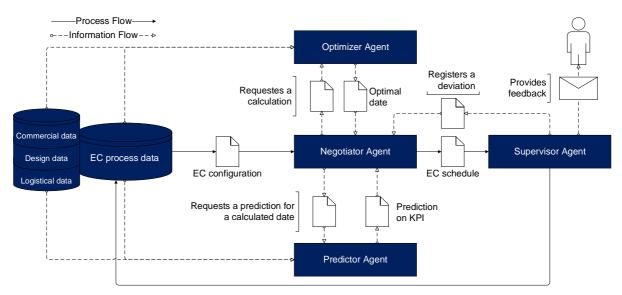
Figure 3. Schematic overview of the role model of the proposed multi-agent system for EC implementation
