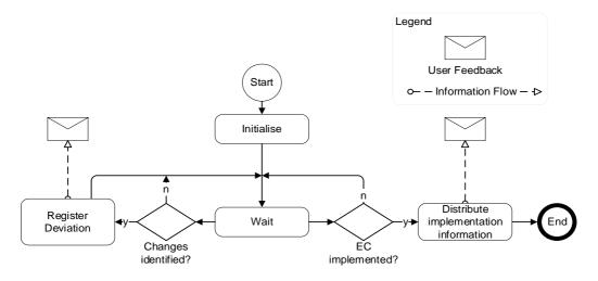
Figure 7. Logic architecture of the 'Supervisor Agent'
