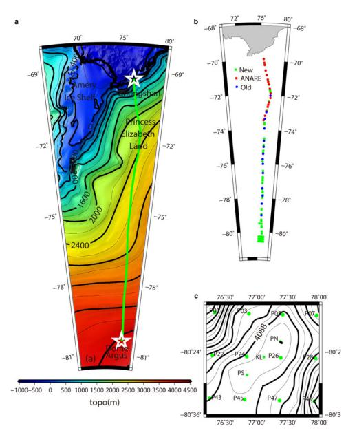
Fig. 1. (a) Sketch map showing the locations of along the transect, and (b) poles for GPS measurements along the transect, and (c) poles for GPS measurements around Dome A.
