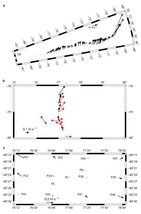
**Fig. 2.** Horizontal ice surface velocity estimates from (a) GPS along the transect, (b) GPS and InSAR along parts of the transect with magnitude  $<5 \text{ m a}^{-1}$ . Red is InSAR, and Black is GPS estimates, respectively, and (c) GPS around Dome A.
