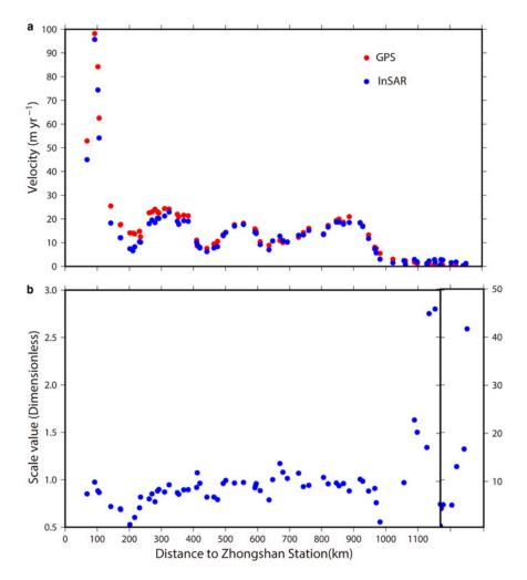
Fig. 3. (a) GPS and InSAR surface velocity along the transect, (b) the factor value derived as the ratio between InSAR surface velocity and corresponding GPS surface velocity.
