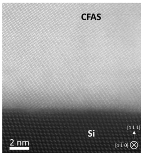
**Figure 1.** Atomic resolution HAADF STEM image at the interface showing the  $\text{Co}_2\text{FeAl}_{0.5}\text{Si}_{0.5}$  film uniformity and structural abruptness of the interface. The imaging is performed along the Si  $[1\bar{1}0]$  zone axis.
