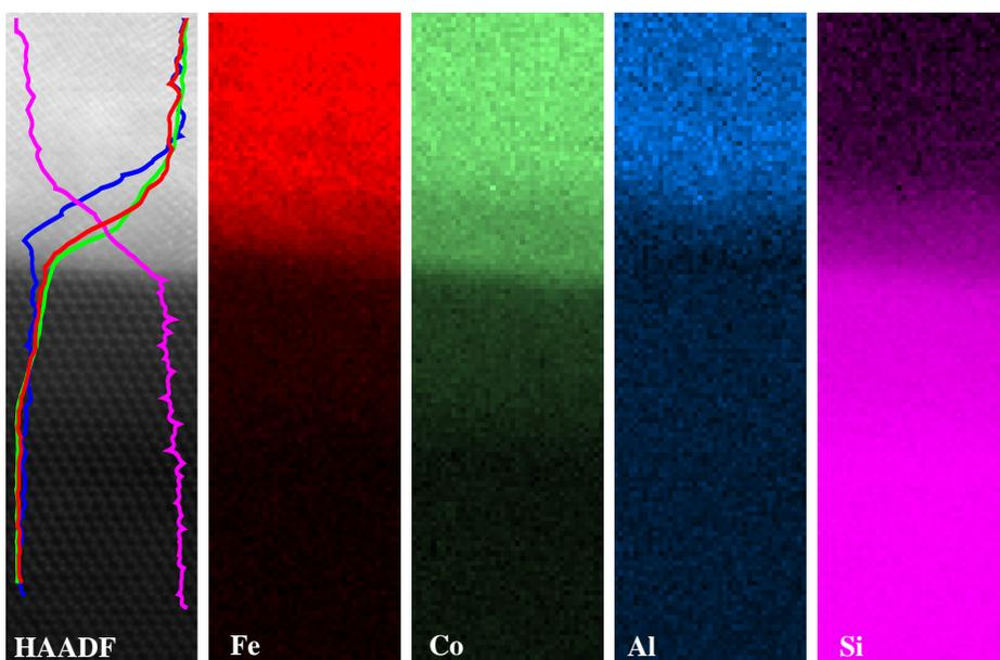
**Figure 2.** HAADF STEM signal and EELS elemental maps of the  $\text{Co}_2\text{FeAl}_{0.5}\text{Si}_{0.5}$  /Si(111) interface showing Si inter-diffusion into the film. The integrated EELS signal of the EELS maps is plotted as line profiles against the HAADF signal.
