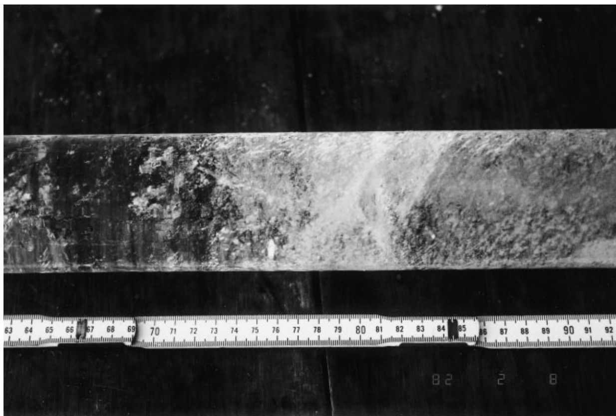
Fig. 6. Hot-water drilled ice core from 1100 m depth showing the transition from bubbly ice at right to clear ice at left.
