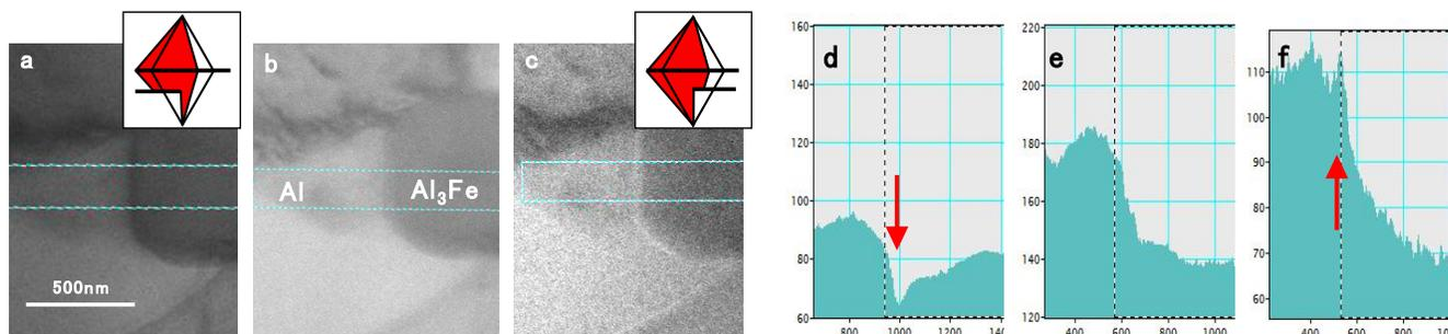
**Figure 3.** BF image of the interface with the aperture in (a) right, (b) without, (c) left hand side, and corresponding intensity profiles (d), (e) and (f), respectively. Insets are the schematic drawing of geometrical optics of the deflected beam with the aperture.
