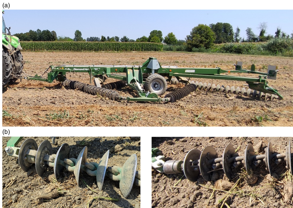
Figure 1. (a) The disc chain harrow Kelly Diamond 1204. (b) Detail of the CL1 discs (left) and K4 discs (right). In Figure 1A, the disc chain harrow is equipped with K4 front and CL1 rear.
