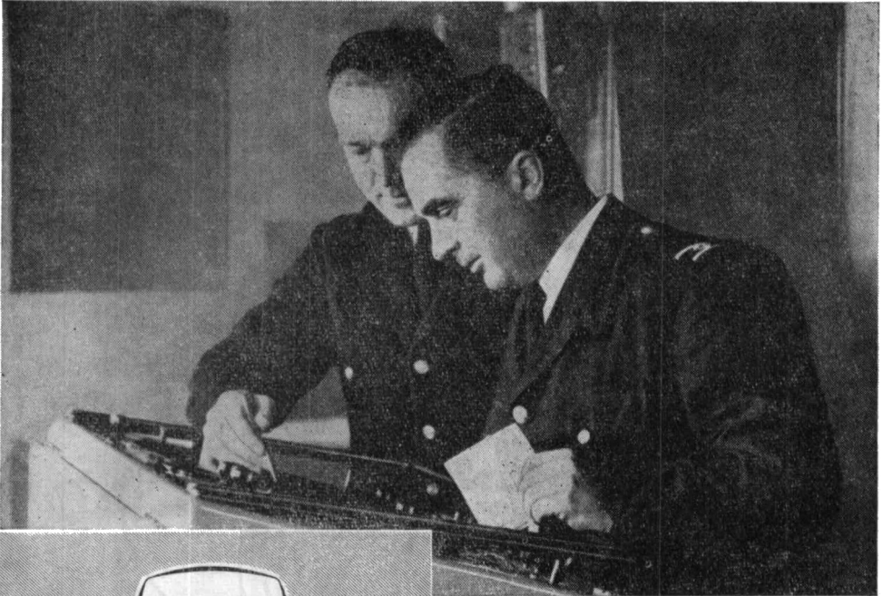
Type 14/16P (True Plot) Display Unit in m.v. 'Pennyworth'. This Unit incorporates a 16-inch P.P.I. display with relative motion or true motion presentation, and built-in reflection plotter.
