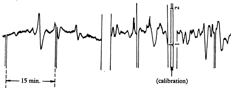
Fig. 1. Two examples of solar scintillation at 140 Mc/s. (21 July 1953).
