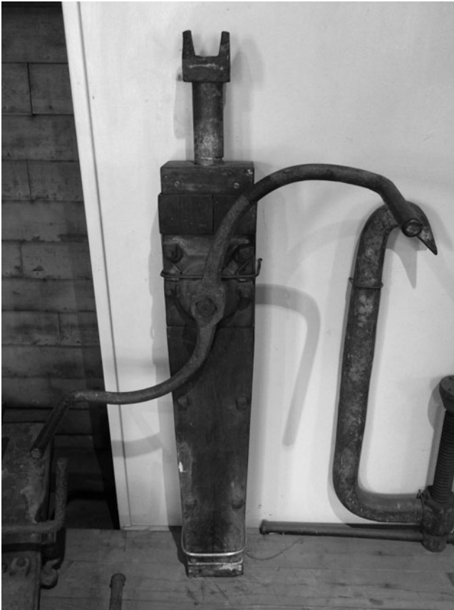
Figure 2. Planking jackscrew, smaller yet similar in operation to the jackscrew used for screwing cotton. Maine Maritime Museum, Bath, ME. Courtesy: the author.
