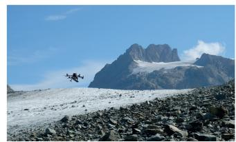
**Figure 1.** Drone-based GPR system: (a) illustration of the system components; (b) diagram showing the structure and interactions between the devices; (c) photo of the system operating over the Otemma glacier in August 2022.
