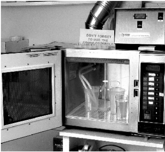
Figure 1a. Original microwave model 3450 series without wattage control or cold spot.
