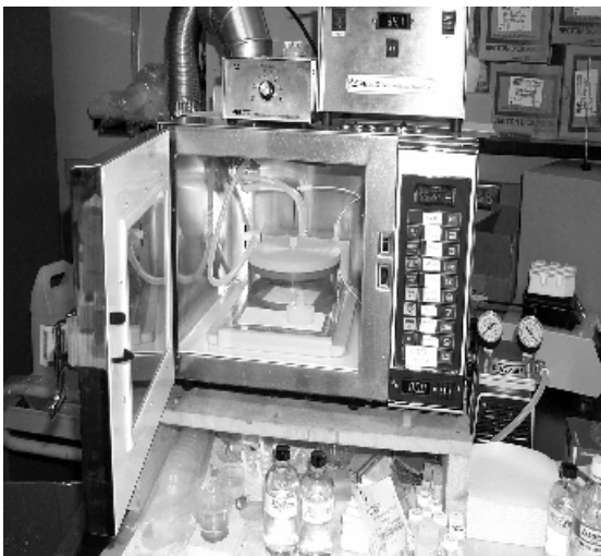
Figure 2a. The newer version of the model 3450 series show variable wattage control unit and cold spot, with vacuum chamber in place.
