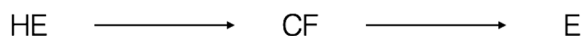
Figure 1. Release of chemicals, represented by E, depended on a component failure, CF, and a human error, HE. The values these variables take on are associated with the occurrence of the respective associated behavior in the system.
