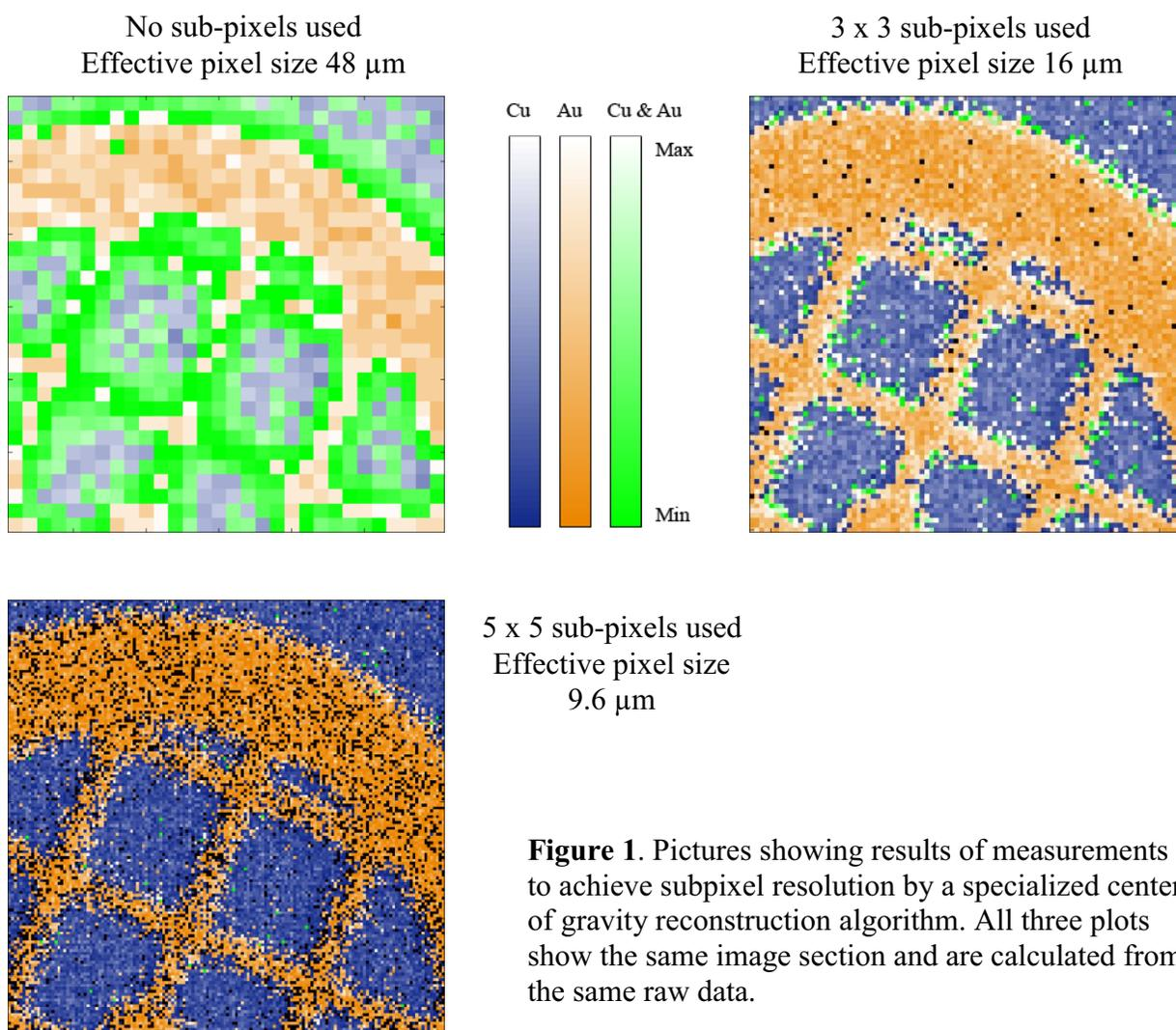
**Figure 1.** Pictures showing results of measurements to achieve subpixel resolution by a specialized center of gravity reconstruction algorithm. All three plots show the same image section and are calculated from the same raw data.
