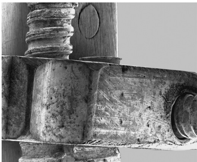
Figure 6: Microscope from Delft canal. Details of the metal shaping can be studied on this image of the stage block. The screw thread shows it was rolled and not cut using modern die techniques; this may be diagnostic of a genuine Leeuwenhoek microscope. The slight splaying of the positioning screw (above center) and the detail of the filed-down rivet head (top center) disclose Leeuwenhoek's diligence.
