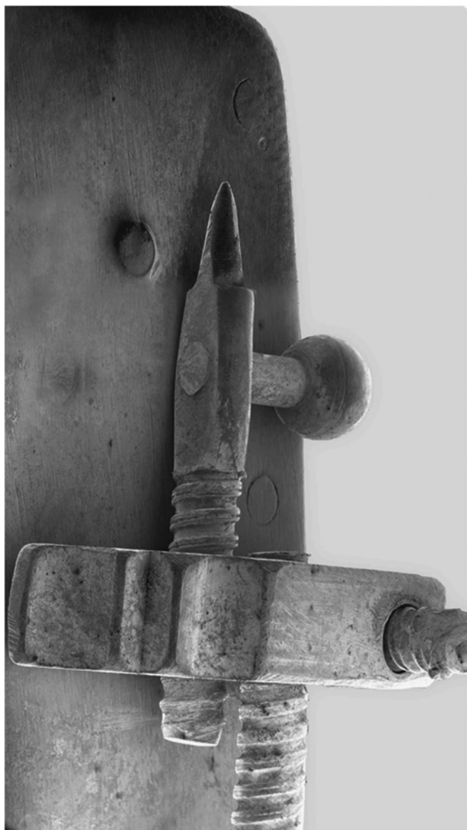
Figure 4: SEM macrograph of the microscope from the Delft canal. A crew from the British program News At Ten filmed studies with the Hitachi S-3400N variable-pressure SEM at the Cavendish Laboratory, Cambridge. We demonstrated that macrographs could reveal fine manufacturing details. This example shows the block stage (below), the abraded lens (upper left) and the specimen pin (center) with its positioning knob.
