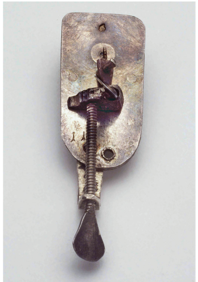
Figure 1: Much media interest in Leeuwenhoek followed my discovery of his specimens in 1981 [2], and this microscope was subsequently brought into the Boerhaave Museum in Leiden, Netherlands. It is the smallest of them all; the plates measure 17×34 mm. It was locked away in the museum for twenty years until it became the subject of a single paper in an obscure journal in 2002 [6].
