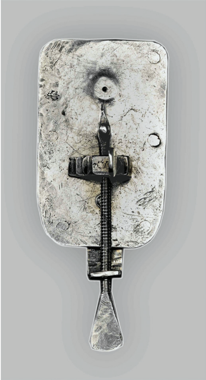
Figure 2: This silver instrument was the first of two identified by the author in 2014. It appears to be a genuine Leeuwenhoek microscope and had been found in a box of toy trinkets. There are air bubbles in the lens, as in some other Leeuwenhoek microscopes. It was never offered for public sale but was sold privately to a Dutch collector.
