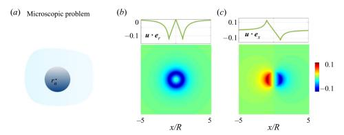
FIGURE 3. Solution of the microscopic problem – a single bubble with pressure  $p_{\infty}$  at infinity (a). Radial velocity (b) and velocity along the x-axis (b) in m s<sup>-1</sup> for an incident plane wave at oblique incidence in the linear regime with amplitude  $\Delta p = 0.1 p_{eq}$ , see main text.
