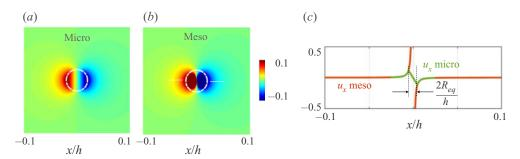
FIGURE 5. Micro-to-meso matching – the solution at the mesoscopic scale is the limit of that at the microscopic scale when  $2R_{eq}/h$  vanishes. Two-dimensional fields of the  $u_x$  velocity at the microscopic scale (a) and at the mesoscopic scale (b); the dotted white lines show the bubble boundary; velocity profiles along the centreline (c).
