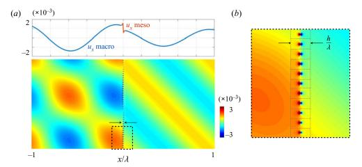
FIGURE 6. Meso-to-macro matchings – the solution at the macroscopic scale for  $x/\lambda \to 0$  is the limit of that of the mesoscopic scale for large x/h; the solution at the mesoscopic scale accounts for the jump in the velocity (2.5). Profiles and fields of the solutions (a); panel (b) shows a zoom near the screen. The incident wave is a plane wave at incidence  $45^{\circ}$  and  $\omega = 0.7\omega_{M}$ .
