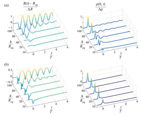
FIGURE 8. Time variations of the radius R(t) and acoustic pressure p(0, t) in (2.5) for increasing array spacing  $h/R_{eq}$  (a) in the linear regime,  $\Delta p/p_{eq} = 10^{-3}$  and (b) in the nonlinear regime,  $\Delta p/p_{eq} = 15$ ;  $\Delta R = (\Delta p/3\gamma p_{eq})R_{eq}$  is the amplitude of linear undamped oscillations.
