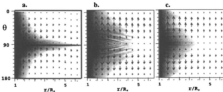
Figure 2. Greyscale of  $\log(\text{density})$  vs. radius and latitude. The superposed vectors show sense and magnitude of latitudinal velocity, with maximum length corresponding to a speed of 100 km/s. The three cases represent models with nonradial line-forces (a) ignored; (b) fully included; (c) computed without latitudinal velocity gradients ( $\partial v/\partial\theta = 0$ ).
