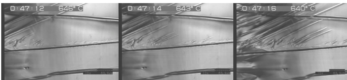
Figure 3. Austenite decomposition Fe-0.18wt%C alloy, with Widmanstätten plates growing from a grain boundary allotriomorph.
