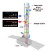
in structural and functional materials microstructure such as dislocations, impurity particles, grain boundaries, and phase boundaries with ~15 ns temporal resolution. Using a specially designed liquid stage, the DTEM also enables observation of live biological processes in real-time with submolecular resolution.
