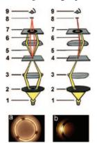
Luminance contrast is a new illumination technique in light microscopy in which the illuminating light, the background light, and the imaging light are totally or partially separated from each other and can be regulated with regard to their brightness and color. The technique is carried out with mirror lenses or modified glass lenses and specialized condensers.
