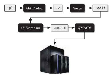
Fig. 5. Overall QA Prolog processing flow.
