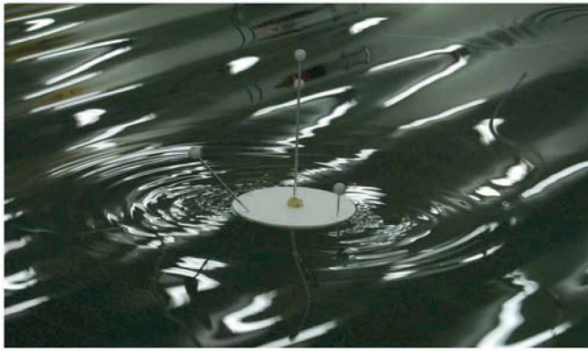
Fig. 2. Model floe during test. Scattered waves are evident.
