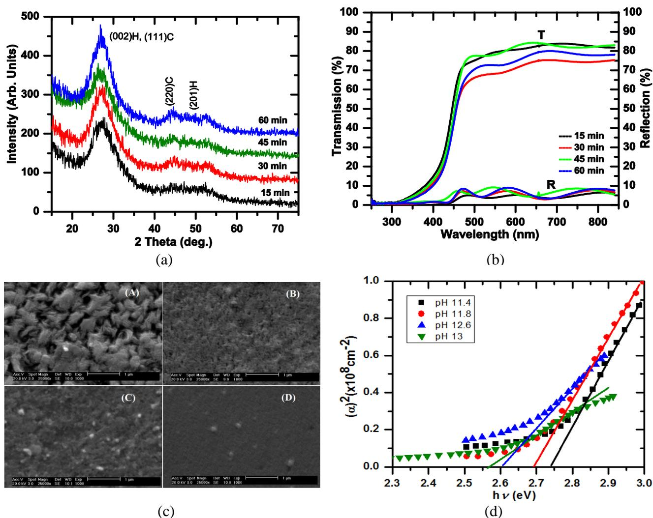
**Figure 1.** X-ray spectrum of a typical CBD-CdS/ZnS sample (a). The transmittance at the high-energy region extends up to 300 nm (b). SEM photos of the samples surfaces of Cd/ZnS films grown at 60 minutes time deposition and to different solution pH, A:11.4, B:11.8, C:12.6 and D:13 (c).  $\alpha^2$  versus  $h\nu$  plot of CdS/ZnS films (d).
