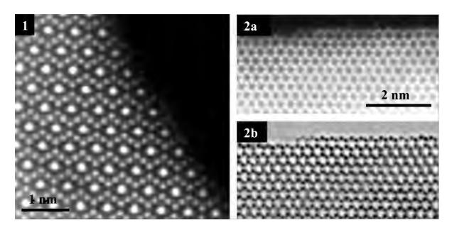
**Figure 1.** Sub-angstrom resolution image of an Fe<sub>3</sub>O<sub>4</sub> nanoparticle, oriented close to the [110] zone axis, clearly reveals the two types of the Fe columns and the reconstruction of the surface Fe atoms. **Figure 2.** HAADF (a) and BF-STEM (b) images of the edge of a hexagonal ZnO plate, oriented close to the ZnO[0001] zone axis. Both the atomic number contrast HAADF and the phase contrast BF-STEM images show the surface atomic arrangement of the ZnO nanoplates.
