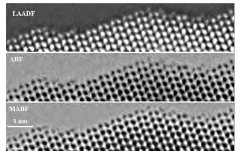
**Figure 3.** Low-angle ADF (LAADF), ABF, and medium-angle BF (MABF) images of a faceted ZnO nanowire. The ZnO nanowire was oriented close to the [11-20] zone axis. Both the LAADF and the ABF images show the oxygen columns, especially at the thinner regions of the nanowire. Surface reconstructions along the different facets are also discernible.
