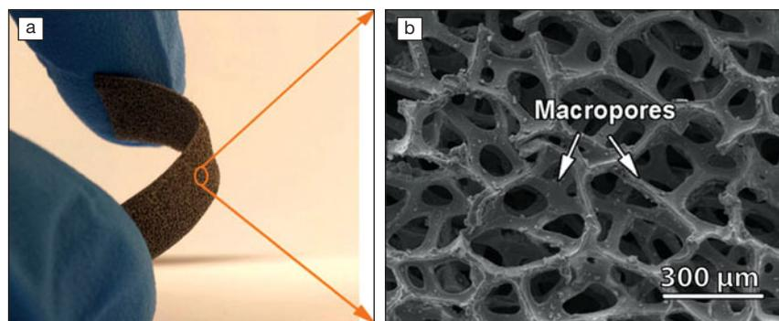
(a) Optical and (b) scanning electron microscope image of the 2D nickel/iron metal-organic framework. Courtesy of Nature Publishing Group.
