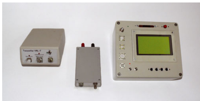
Fig. 2. View of the radar system elements. The TX subsystem is shown on the left and the two units of the RX subsystem are shown in the centre (RA) and on the right (CRU).
