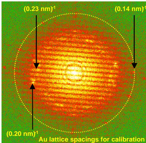
**Fig 2:** Information limit of the FEG TEM measured by means of Young fringes. Reflections from gold clusters on the amorphous carbon foil can be used for calibration. Linear information transfer down to below
