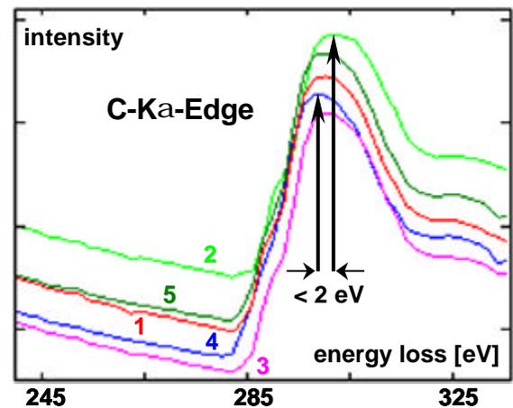
**Fig 1:** *Left:* Energy loss image of holey carbon foil taken with 2 eV energy width at the C K $\alpha$ -edge. *Right:* Energy spectra extracted out of a series of energy loss images from the marked areas. Within the field of view of 2.5 μm an energy shift <math>< 2 \text{ eV}</math> is apparent.
