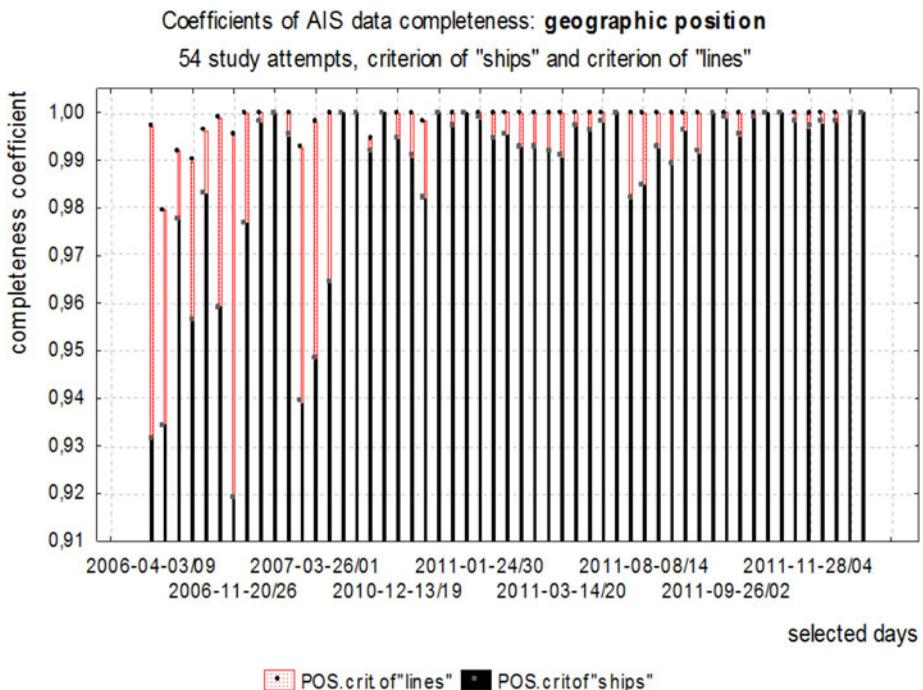
Figure 16. Geographical position coefficients of AIS data completeness.
