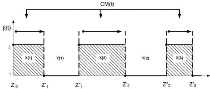
Figure 8. Graphic presentation of completeness of AIS data (Specht C., 2003).where:  $CM(t)$  – completeness of AIS data;  $\beta(t)$  – system state;  $X(n)$  – working time;  $Y(n)$  – time of failure.
