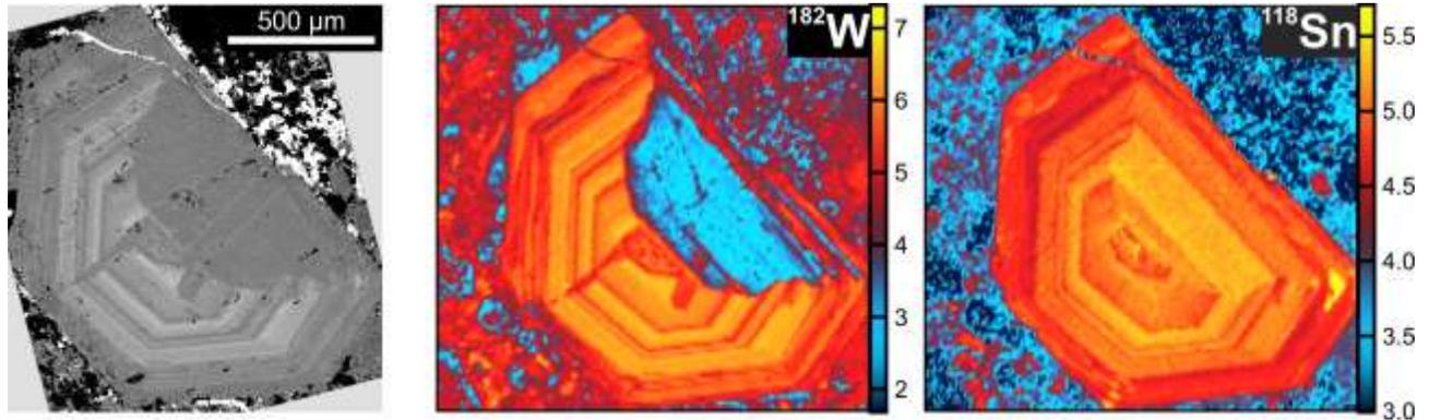
**Figure 1.** BSE image and LA-ICP-MS maps of zoned hematite grain. Scale in cps (log 10<sup>n</sup>) [5]
