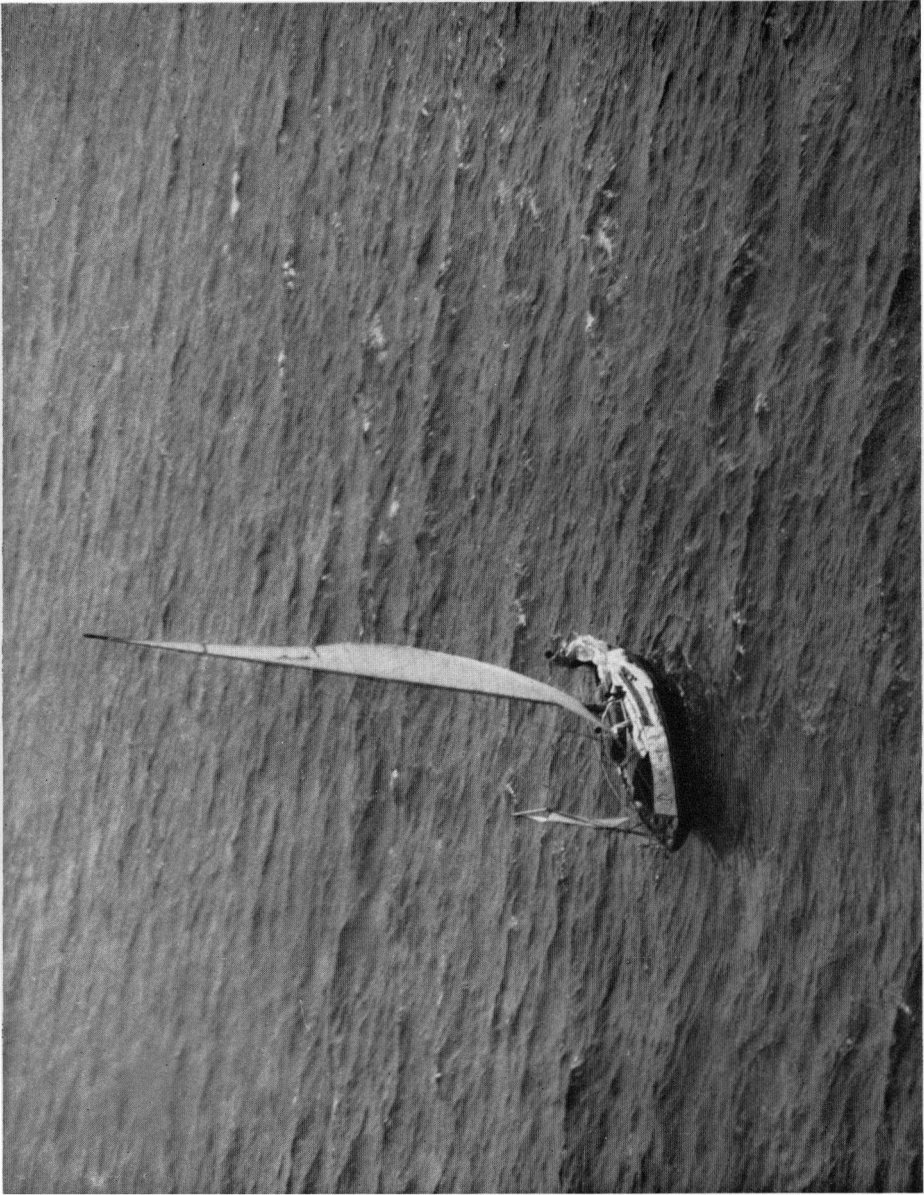
Francis Chichester's Gipsy Moth III at the finish of the single-handed transatlantic race. The 45-square foot mizzen weather-cocks with the wind and controls the tiller.
