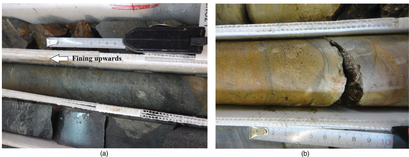
Fig. 12. A. Greenish-grey and coarse-grained greywacke drill cores of RGM. B. Scours at the bottom of the layers in the drill cores of RGM.
