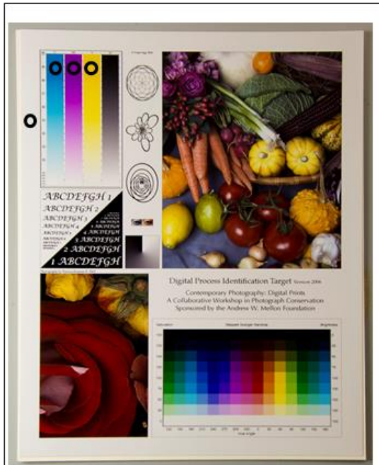
Fig. 1. Sample of an 21.59 cm by 27.94 cm chromogenic photograph which is a 2007 version of the American Institute for Conservation-Photographic Materials Group (AIC/PMG) Digital Print Sample Set with the selected regions of interest (in circles) that was microfade tested for unmounted and face-mounted photographs.
