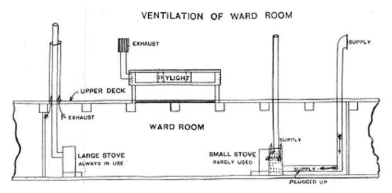
Figure 1. Ventilation System Employed on the Discovery. A similar system was employed in the crew's living quarters. Scott, The Voyage of the Discovery, 1: 342.
