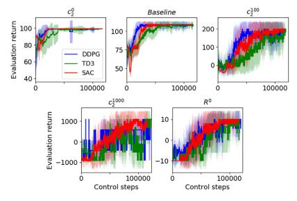
Figure 12. Ensemble average and standard deviation of the evaluation return computed with only trials that led to a winning test trajectory (the average may therefore be performed with different number of runs for each algorithm). The curves were obtained by evaluating the policies at the end of each episode during training.
