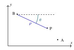
*Figure 4.* Airfoil polar coordinates  $(\rho, \theta)$  defined relative to point B.
