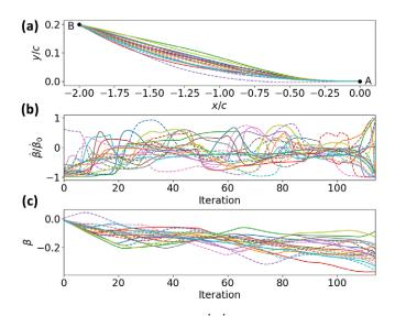
**Figure 10.** (a) Trajectory, (b) normalized action  $\beta/\beta_0$ , and (c) pitch angle  $\beta$  obtained by testing 20 identically parametrized agents. Returns from all the tests are in the range [109.12; 109.58]
