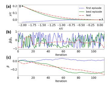
*Figure 9.* (a) Trajectory, (b) normalized action  $\beta/\beta_0$ , and (c) pitch angle  $\beta$  for three selected episodes of the training and testing: the first and best episode (i.e., with the highest return) of training and the test episode. Corresponding returns are respectively equal to 80.99, 109.78, and 109.69.
