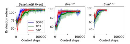
**Figure 18.** Ensemble average and standard deviation of the evaluation return computed with only trials that led to a winning test trajectory (the average may therefore be performed with different number of runs for each algorithm). The curves were obtained by evaluating the policy at the end of each episode during training.
