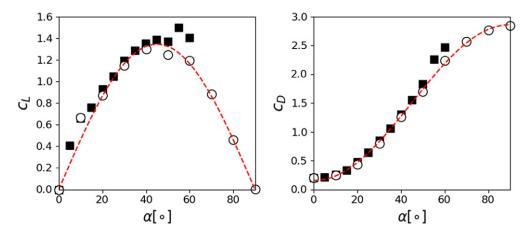
**Figure 3.** Evolution of the lift  $c_L$  and  $drag c_D$  coefficients with the angle of attack  $\alpha$ . Results from Taira and Colonius (2009) ( $\blacksquare$ ), present study using STAR-CCM+ ( $\circ$ ), and fitting of the present study data using Eq. (3) (- -).
