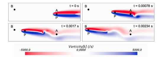
**Figure A1.** Instantaneous vorticity field at various time steps of the CFD-DRL framework applied to the trajectory control of an airfoil going from point A to point B. The action sequence of this maneuver is obtained by testing one of the 20 policies obtained for the 20 trials performed with SAC for the CFD case discussed in Section 4.4.
