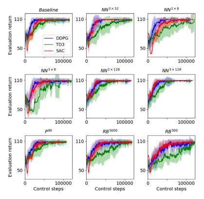
**Figure 11.** Ensemble average and standard deviation of the evaluation return computed with only trials that led to a winning test trajectory (the average may therefore be performed with different number of runs for each algorithm). The curves were obtained by evaluating the policy at the end of each episode during training.
