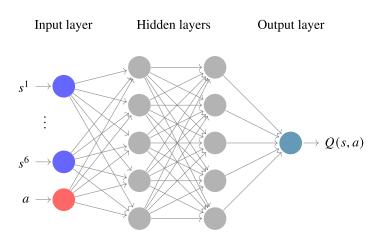
*Figure 6.* Generic architecture of the state-action value function  $Q^{\pi}(s,a)$  neural network.
