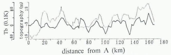
Fig. 7. High-pass filtered variations on surface topography (thin line) and the Tb (thick lines) along the over-snow traverse route in Figure 6(a).
