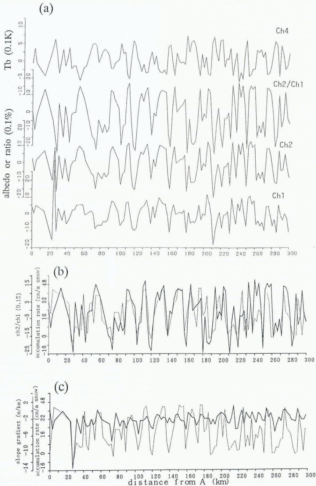
Fig. 5. (a) High-pass filtered profiles in channels 1, 2, 4 and R2/1 along the line in Figure 4b. Units are 0.1% in albedo or R2/1, and 0.1 K in Tb. (b) The relationship between accumulation rate (thin line) and high-pass filtered R2/1 (thick line) along the line shown in Figure 4b. (c) Relationship between accumulation rate (thin) and slope gradient (thick) along the line shown in Figure 4b. Large negative values in the slope mean steep slopes.
