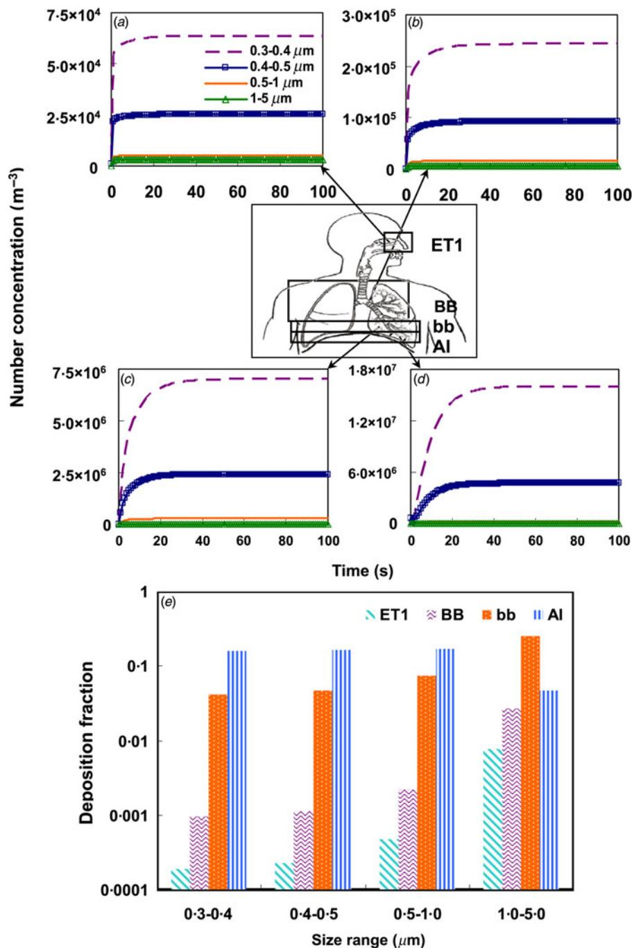
**Fig. 3.** Deposited droplet number concentrations for ranges 0.3–0.4, 0.4–0.5, 0.5–1, and 1–5 μm in (a) ET1, (b) BB, (c) bb, and (d) AI regions, respectively. (e) Human respiratory tract region-specific deposition fractions for 0.3–0.4, 0.4–0.5, 0.5–1, and 1–5 μm, respectively.
