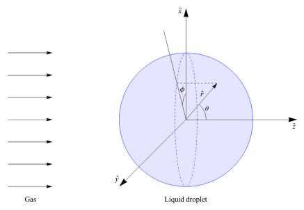
Figure 1. Schematic of a rarefied gas flow past a spherical liquid droplet.
