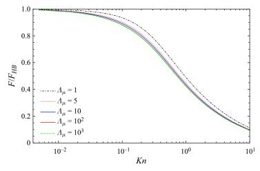
Figure 3. Drag force on the liquid droplet normalised with the drag force given by (4.9). The thermal conductivity ratio is  $\Lambda_{\kappa} = 100$ .
