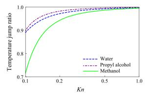
Figure 15. The ratio of the temperature jump at the interface of a liquid droplet (made of water, propyl alcohol and methanol) to the temperature jump at the interface of a corresponding solid sphere  $(\Lambda_{\mu} \to \infty)$  having the same thermal conductivity as that of the liquid against plotted over the Knudsen number.
