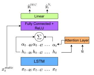
**Figure 2.** Architecture of the LSTM-based model with integrated attention method to predict IWC and  $N_i$  of cirrus clouds with the temporal data set. ReLU, rectified linear unit.
