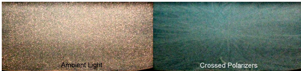
Figure 1. Examples of unpolarized (left) and cross-polarized imaging (right) of the same piece of foam.
