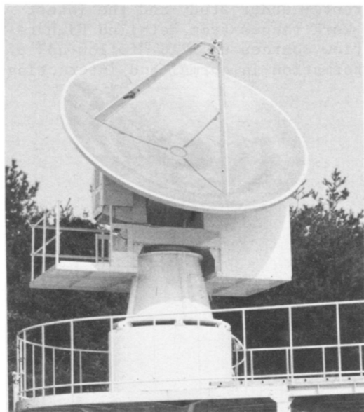
Fig. 1. The 4-m millimeter wave telescope at the Department of Physics and Astrophysics, Nagoya University.
