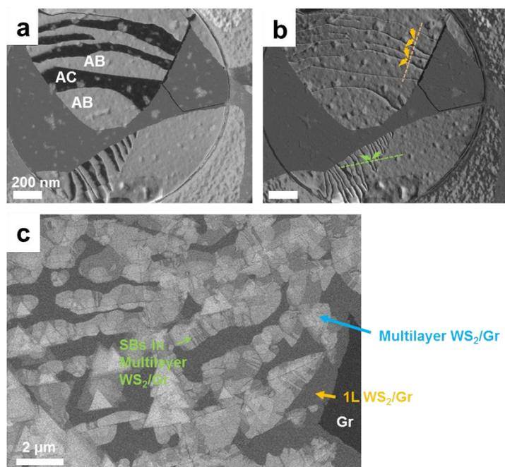
**Figure 1.** (a-b) Dark-field TEM images obtained by (a)  $(0\bar{1}10)$  (1<sup>st</sup>) and (b)  $(\bar{2}110)$  (2<sup>nd</sup>) diffraction spots, respectively. (a) and (b) indicate stacking order and layer number, respectively. Orange and green arrows in burgers vector of partial dislocations using adjacent 2<sup>nd</sup> order dark-field images. (c) SEM image using backscattered electron mode, showing stacking order. SBs are formed near the graphene wrinkles.
