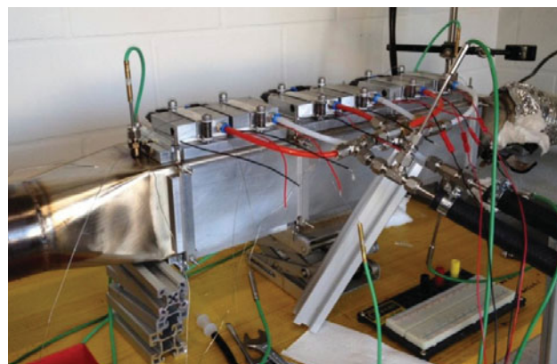
Thermoelectric converter tests on a methane/hydrogen motor of a customized hybrid vehicle—CCEM project cohyb—delivered 120 W electricity, which equals to 3% fuel saving. Credit: EMPA.
