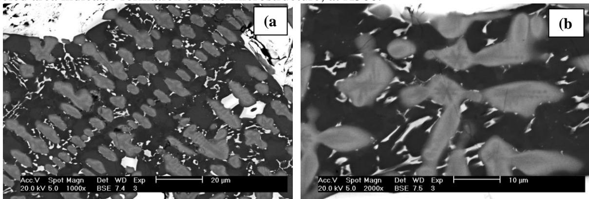
**Figure 2.** BSE images of typical microstructure of the centre of the cast alloy, a) The  $Al_3Nb$  dendrites, at X1000, b) Details of fine microstructure which consisted of  $Al_3Nb$ ,  $\tau$  and  $Ti_5Si_3$  phases, at X2000.
