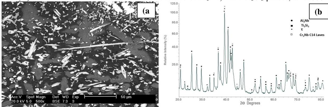
**Figure 3.** a) BSE image of typical microstructure in the bottom of the cast alloy, the  $Ti_5Si_3$  silicide presented a finer microstructure and a lower volume fraction, at X500, b) XRD diffractogram of the alloy powder showing the phases present in the cast condition.
