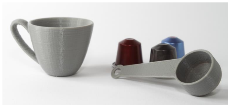
Figure 6. Food industry prototype printed using PLA materials (Picture from: https://www.hubs.com/knowledge-base/pla-vs-abs-whats-difference/ )
