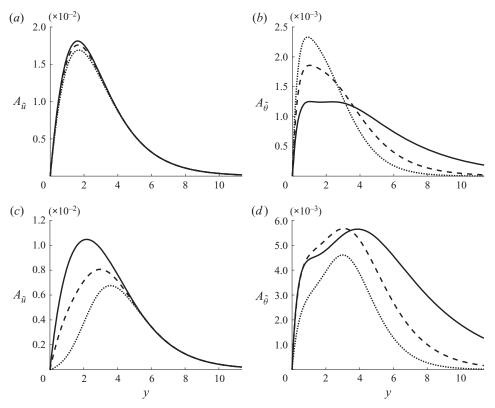
Figure 4. The amplitude of the velocity streaks (a,c) and thermal streaks (b,d) for Prandtl number  $\sigma = 0.71$  (solid black line), 1 (dashed line) and 1.3 (dotted line). The amplitudes in (a,c) are for a subsonic free-stream Mach number  $M_{\infty} = 0.8$  whilst (b,d) are for the moderate supersonic regime with  $M_{\infty} = 2$ . The Reynolds number is  $Re = 80\,000$  and we have used  $\zeta = 0.76$  in the power-law viscosity law (3.7) to calculate the basic flow.
