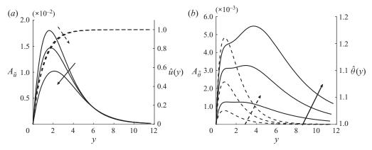
Figure 3. The amplitude of the velocity streaks (*a*) and thermal streaks (*b*) (solid lines, left axis), together with the basic flows  $\hat{u}(y)$  and  $\hat{\theta}(y)$  (dashed lines, right axis) for free-stream Mach numbers  $M_{\infty} = 0.8$ , 1.4 and 2. The arrow indicates the direction of increasing Mach number. The Prandtl number is  $\sigma = 0.71$  and we have used  $\zeta = 0.76$  in the power-law viscosity law (3.7) to calculate the basic flow.
